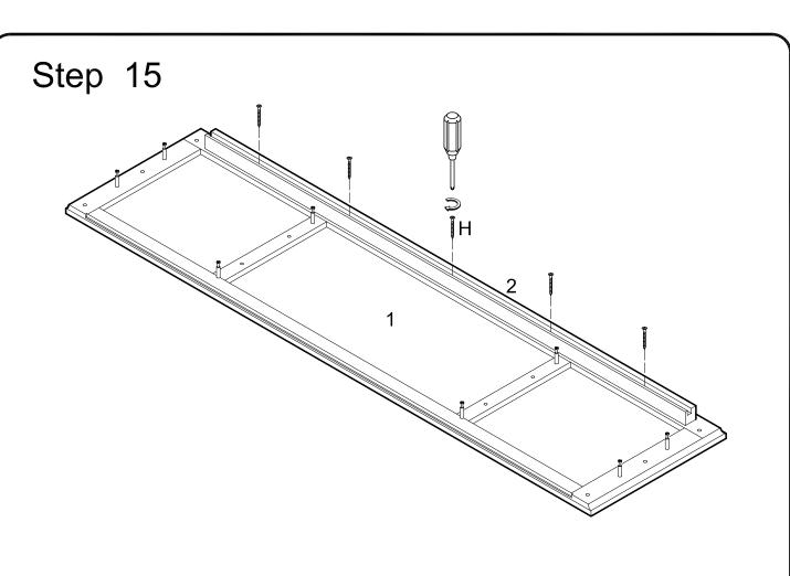
Attach slat (2) to top panel (1) using screws (H).
